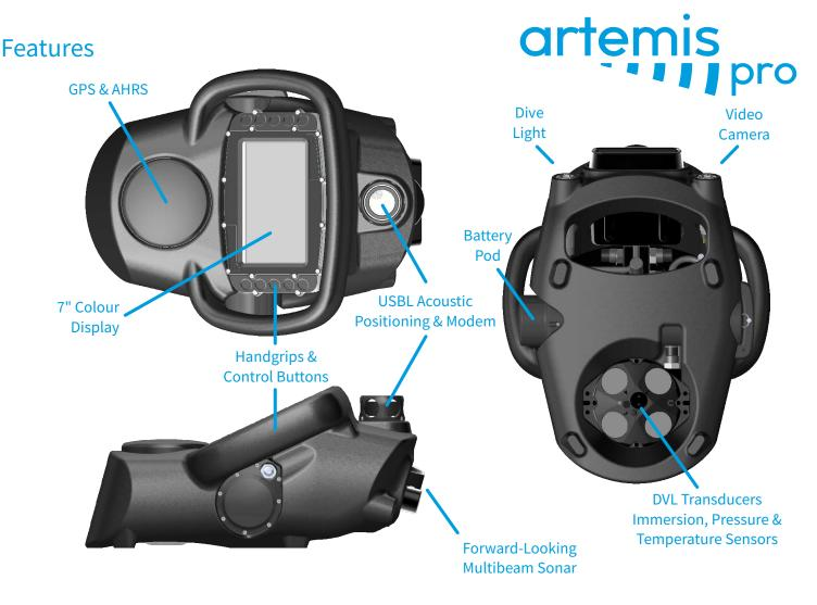
**ARTEMIS PRO is intuitive and straightforward to use.** The interface has been designed by divers for divers. The user can quickly interpret information presented via the simple menu interface and graphical display, and easily switch between Sonar, Navigation and other displays with the touch of a button.
