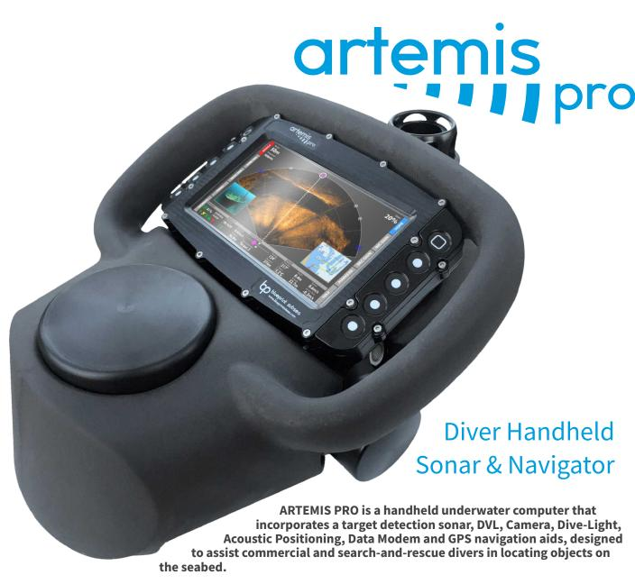
ARTEMIS PRO has also been specifically optimised for use by Naval Mine Clearance, EOD and Commercial Divers for locating and navigating to submerged targets as an alternative to conducting a tactile or circular search around a known datum, or large area survey work to identify objects on the seabed.
