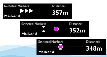
If the diver is more than 30°, 60° or 90° off the desired heading, 1, 2 or 3 arrows indicate respectively that they should turn either left or right. Below 30°, a circular 'bubble' moves across the status bar to allow fine tuning of the course.
