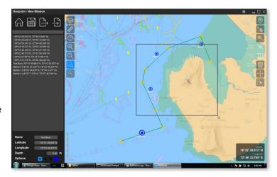
During a dive, ARTEMIS PRO will collect and record all the sensor information received from the Sonar, GPS, DVL, internal compass and depth sensor into a Dive Log file.
