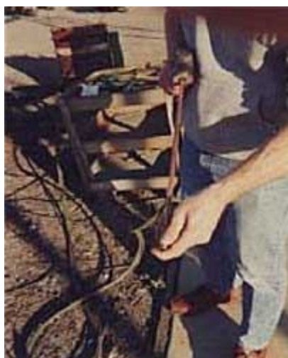
1. Fit RapidFire® igniter cartridge to end of cutting rod..
